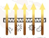
Contaminated air is blown through a HEPA filter and either recirculated (A2) or directed to the duct system (A2/B2)
