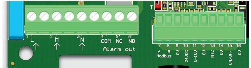
When VentilationAlarm EP2 is used to monitor a voltage signal (0-10V) a minimum and maximum setpoint can be set. Alarm is activated if signal falls under minimum setpoint or exceeds maximum setpoint.
